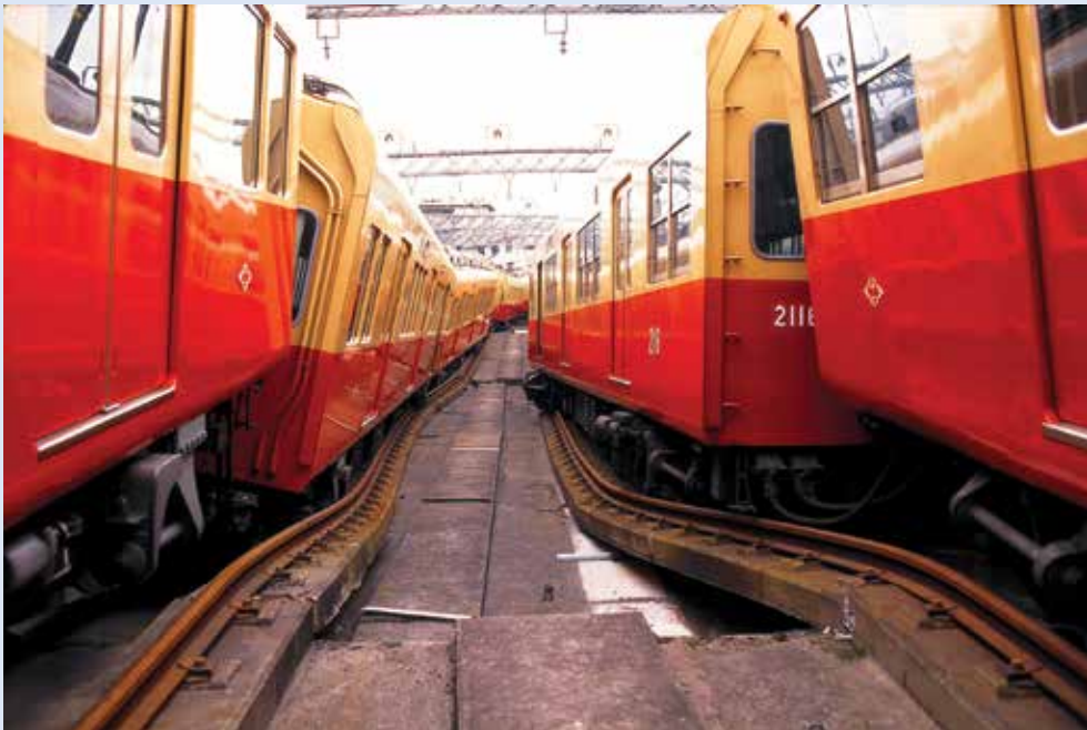
IMAGE B17.4.1. Trains Parked at the Shinzaike Depot on the Hanshin Dentetsu Line Thrown to One Side Following the Great Hanshin Earthquake: Japan, 1995
