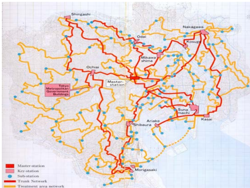
Figure 8.31: Fiber optic cable network in Tokyo's sewage system
