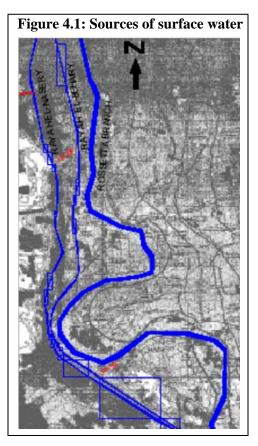
Nasery receives an extra 1.6 Mm3 per day at km 38 through the culvert from the Rayah El Behairy. The Raya el Nasery has two cross regulators to control water flow. The first cross regulator is at km 70.9, the second one is at km 81.5.
